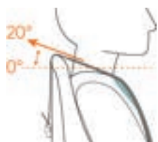
When the top straps are pulled at an upward angle, above shoulder level, shoulder envelopment is reduced.
