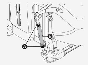
This is the other way to adjust the angle of the armrest.  $\checkmark$  Allen key 5 mm
