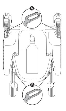
The wheelchair is equipped with four tie-down points used for transportation  $\blacksquare \checkmark \textcircled{B}$ . Two in the front ((a)) and two in the rear ((b)).
