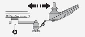
This is how you adjust the resistance of the rotational panel holder. Loosen or tighten knob **(2)** on the friction joint to adjust how easily the rotational panel holder can be pushed to either side.
