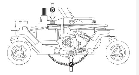
The serial number label is located on the lower, left side of the wheelchair chassis (). An additional serial number label is located on the seat tilt (). You may need to tilt the seat to see the serial number label.
