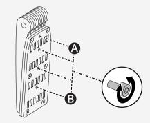
This is how you adjust the height and depth of the headrest.  $\checkmark$  Allen key 5 mm
