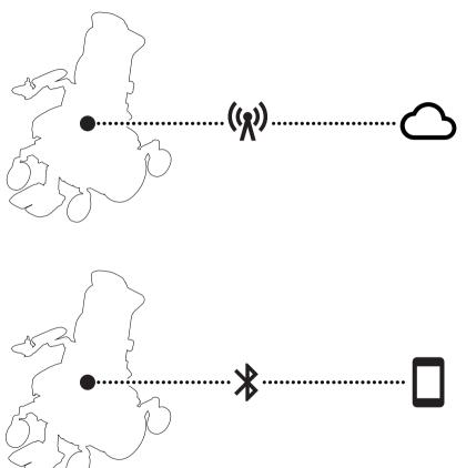
Your power wheelchair has a Power Platform, which contains a radio transmitter. In certain areas, radio transmission is not allowed and your wheelchair must be set to flight mode  $\checkmark$ .
