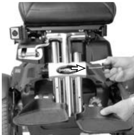
Height adjustment of the foot plates.
