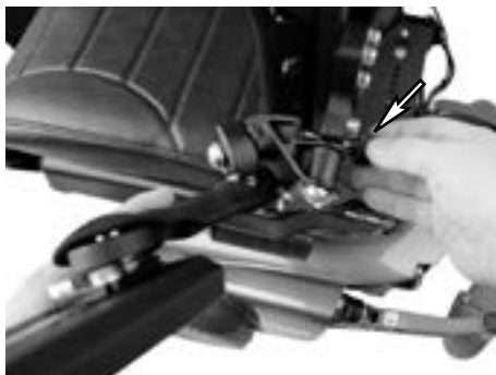
Adjustment knob for angling the arm rest.
