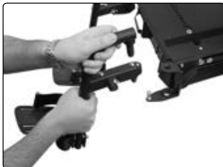
Removing/attaching the leg support
