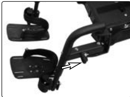
Loosen the catch by push it backwards.
