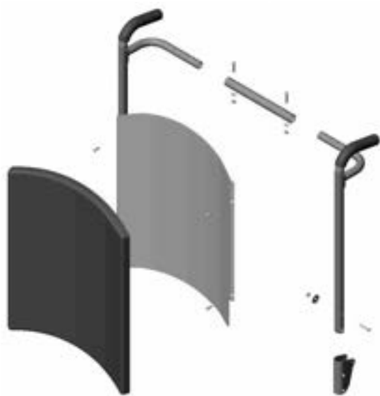
Adjustment of back rest width
