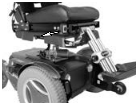
Spring-lock pin for the leg rest angle.
