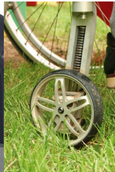
Suspension forks – reduce pain sensitiveness and paroxysmal extensor spasms caused by uneven terrain
